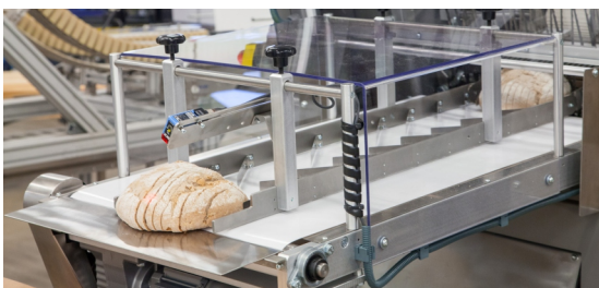
Band conveyor outlet
