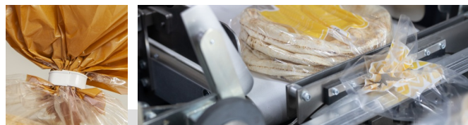
Loafmaster GRP is equipped with integrated clipband closing system
